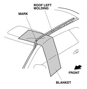
8. Place an empty cardboard box (approx. 120 mm tall) under the roof left molding near the mark.
