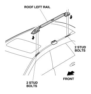
27. Secure the roof left rail to the left center stay with two short Torx bolts. Torque the short Torx bolts to 7-12 N·m (5-9 lbf-ft).
