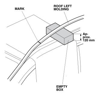
While wearing eye protection, use an air saw to cut the roof left molding at the mark. Do not use a cutting wheel or shears to cut the molding, it will damage the roof left molding. Have an assistant hold the rear edge while cutting.
