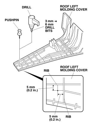
5. While wearing eye protection, drill the pierced mark with a 3 mm drill bit. Enlarge the hole with a 6 mm drill bit. Remove any burrs.
