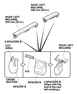
22. Install the four spacers B into the ends of the pieces of the roof left molding.
